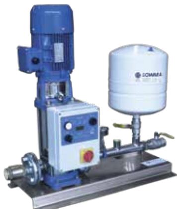
Standard Single Pressure Pac with Stainless Steel manifold, base, pump controller, gauge, NRV, isolation valves, pressure transducer and pressure tank
