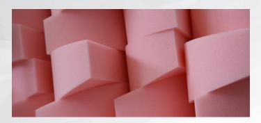
Polyurethane foam is produced when a polyether is treated with a isocyanate in the presence of water and a catalyst, as well as fillers, dispersing and emulsifying agents, etc. The water reacts with the isocyanate group to cause cross linking and curing, and also produces carbon dioxide which causes foaming.
