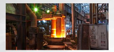
The liquid that remains after the distillation of coal tar or refining of petroleum. It is used in paints, roofing and paving materials. It is also used in the production of graphite anodes for electric arc furnaces used in steel production (shown) and carbon anodes used in electrolytic aluminum smelters.
