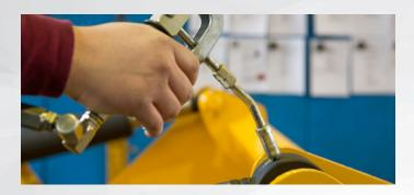
Commonly referred to as lubricating, automotive, or bearing grease. Generally mixtures of a mineral oil with one or more metallic soaps; the most common are those of sodium, calcium, barium, aluminum, lead, lithium, potassium and zinc. The texture of grease may be smooth, buttery, ropy, fibrous, spongy or rubbery. Viscosities range greatly. However, grease is extremely shear sensitive. Typically flow is aided by a follower-plate on the supply tank.
